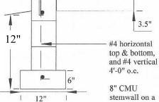
stemwall on a 6" hgt x 12" wide concrete
